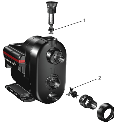
Outlet and inlet non-return valves
